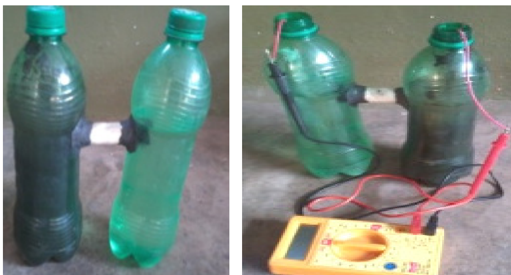
Fig. 1. Measurement of electricity in two chamber containing sewage
