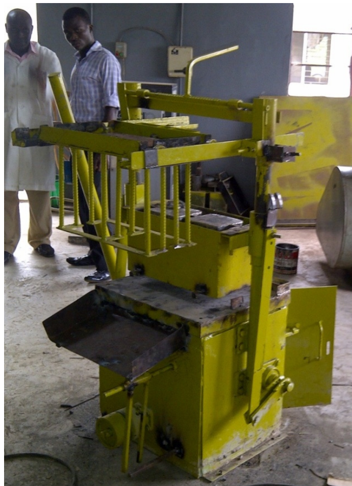
Fig. 6. Picture of the fabricated double mould vibration compactor block moulding machine
