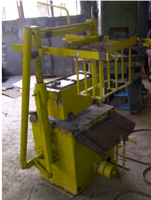
Fig. 7. Pictures showing different side views of the double mould vibration compactor block moulding machine (during fabrication)
