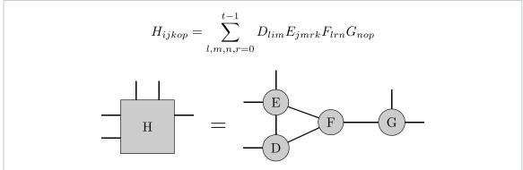
**Figure 1.** Tensor network representing fifth-order tensor *H*, depicted using explicit summations (top) and a tensor diagram (bottom). The network is generated by four different contractions, each of which is indicated in the diagram by a shared leg. While it is possible to discern the contraction pattern of the component tensors by studying the index notation, the diagram makes it obvious at a glance.
