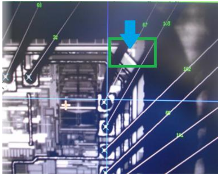
Fig. 5. Adjusted wirebond parameter to J-wire loop, resulting in visible L-fiducial
