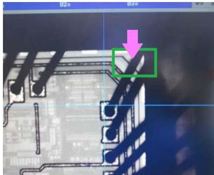
Fig. 2. L-fiducial obstructed after completion of first wirebonding sequence
