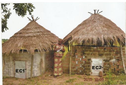
Plate 1. Evaporative coolers 1 & 2 EC1= Non-Cladded Burnt-Clay-Brick Evaporative Cooler (NBEC); EC2=Aluminum-Cladded Burnt-Clay-Brick Evaporative Cooler (ABBEC)
