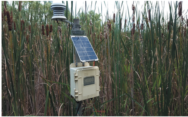
Figure 2. The installation of the HOBO U30 data logger device ( https://www.utm.utoronto.ca/geography/resources/environmental-datasets ).
