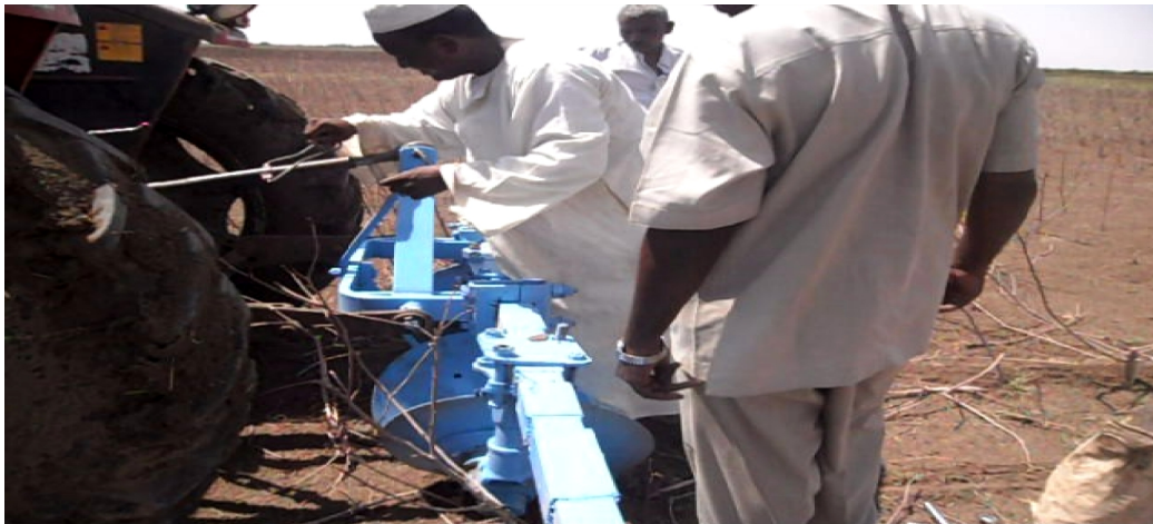
Fig. 3.6B. Adjustment of rake angle
