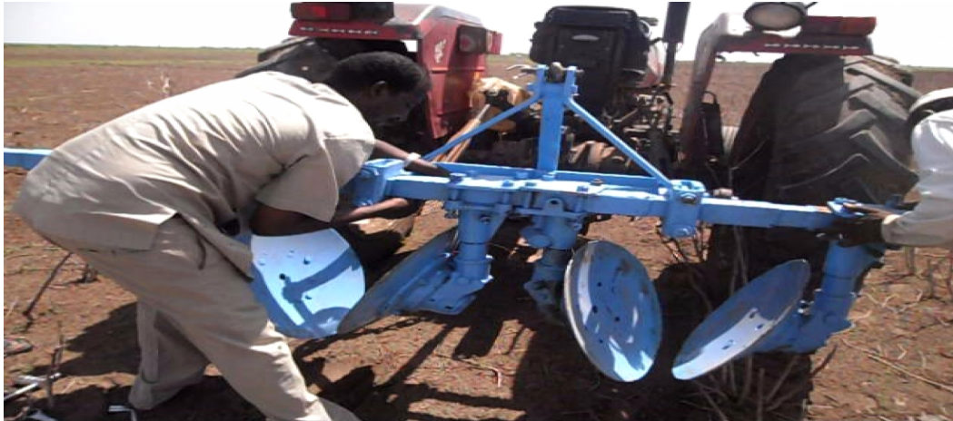
Fig. 3.6A. Adjustment of rake angle
