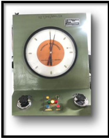
Fig. 9. The load required to debond the specimen was recorded
