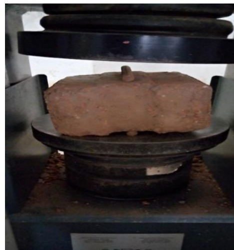
Fig. 9. Tensile test of compressed laterite interlocking blocks
