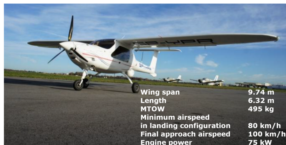
Figure 2. The MP-02A experimental airplane, as used in the research.
